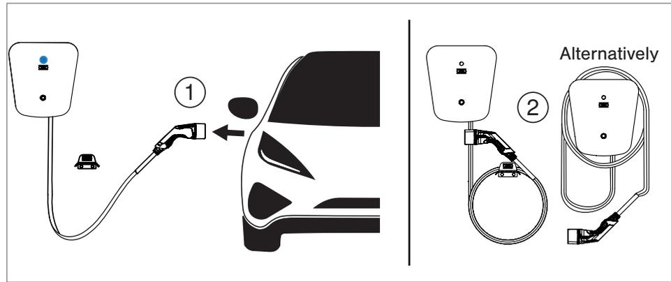
**Fig. 3:** Ending the charging operation
